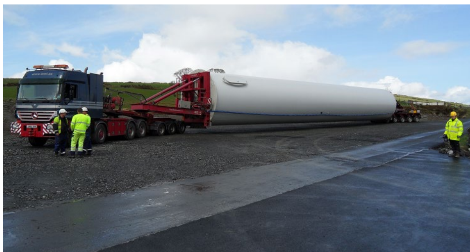
Plate 2.1: Typical Haulage Vehicle for Turbine Delivery
