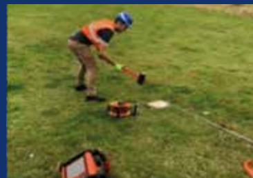
DAM Geotechnical Geophysicist acquiring seismic refraction data.
