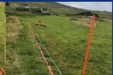
Setting up the electrical resistivity method on L01.
