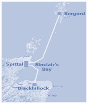
The Viking wind farm will be connected to the UK mainland transmission network by a 600MW HVDC subsea cable connection. The connection will be constructed and operated by SHE Transmission as a regulated network asset in accordance with their licence obligations. The needs case for the project was submitted to Ofgem in October 2018.
