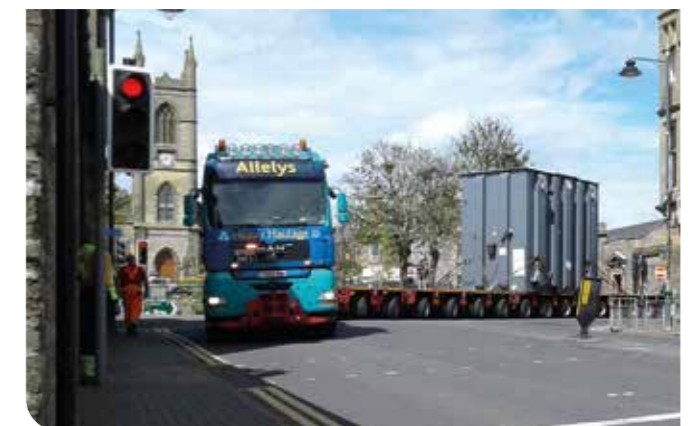
Spittal HVDC transformer being transported through Thurso.
